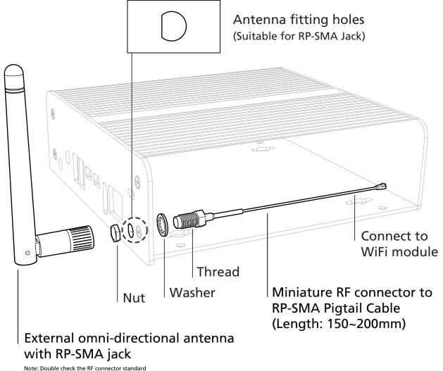
Note: Double check the RF connector standard on your WiFi module prior to sourcing your pigtail cable.
